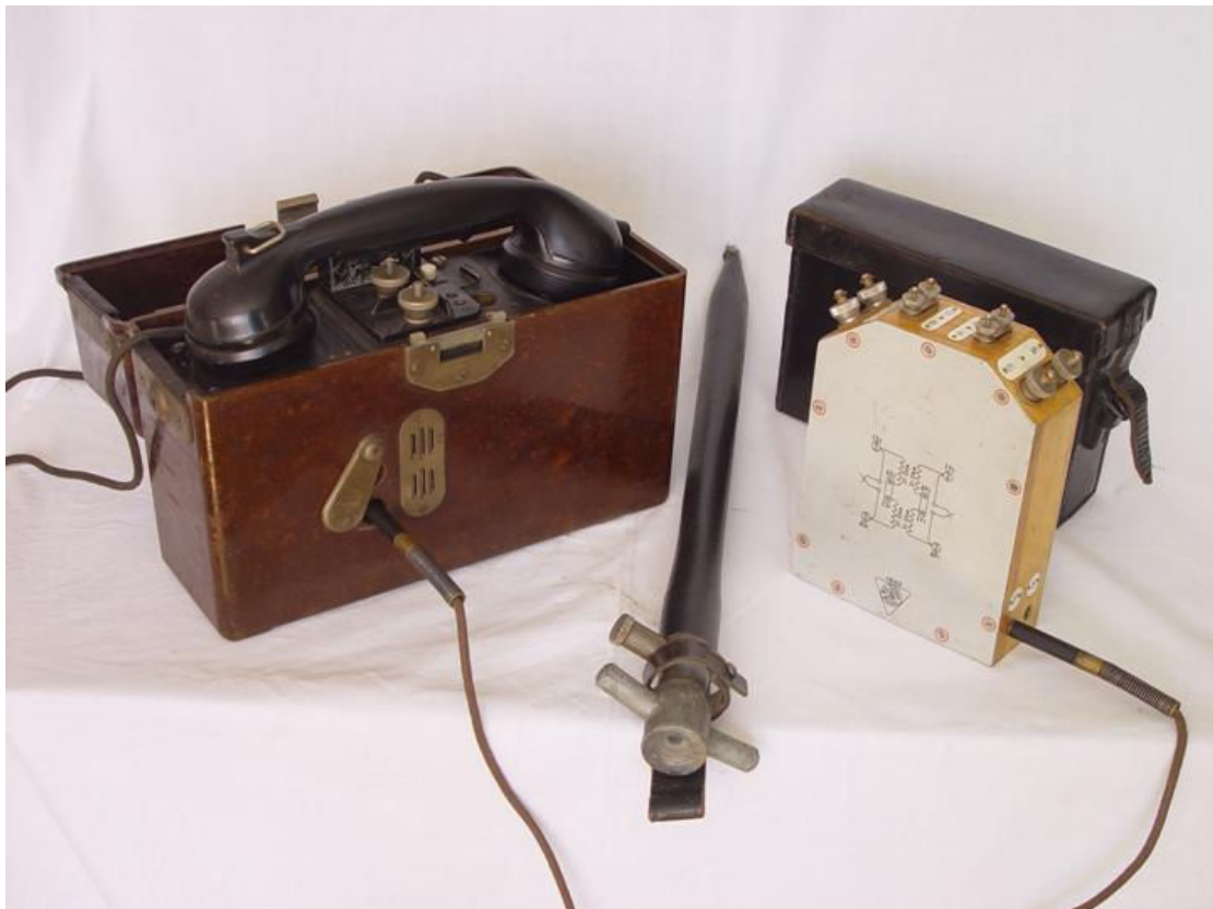
Figure 232: Übertrager connected directly to a FF 33 field telephone
