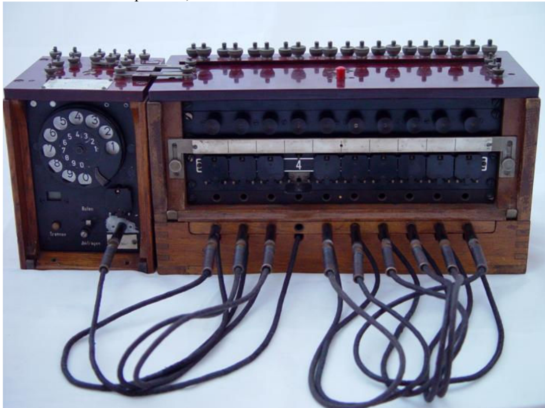
Figure 142: Line 4 of the Klappenschrank connected to an external line
